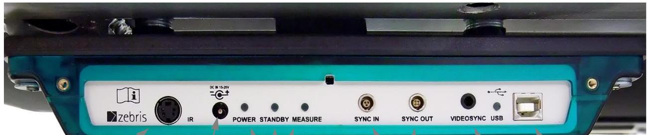
IR-Sync.      Pow-ersupply      Operation Mode Indicator      zebris Sync IN/OUT      Video-Sync.      USB-Socket
