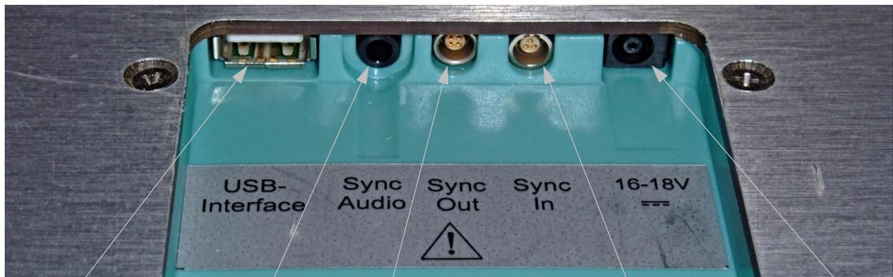
USB-socket      Video-Sync      Sync Out/Master      Sync In/Slave      Power supply
