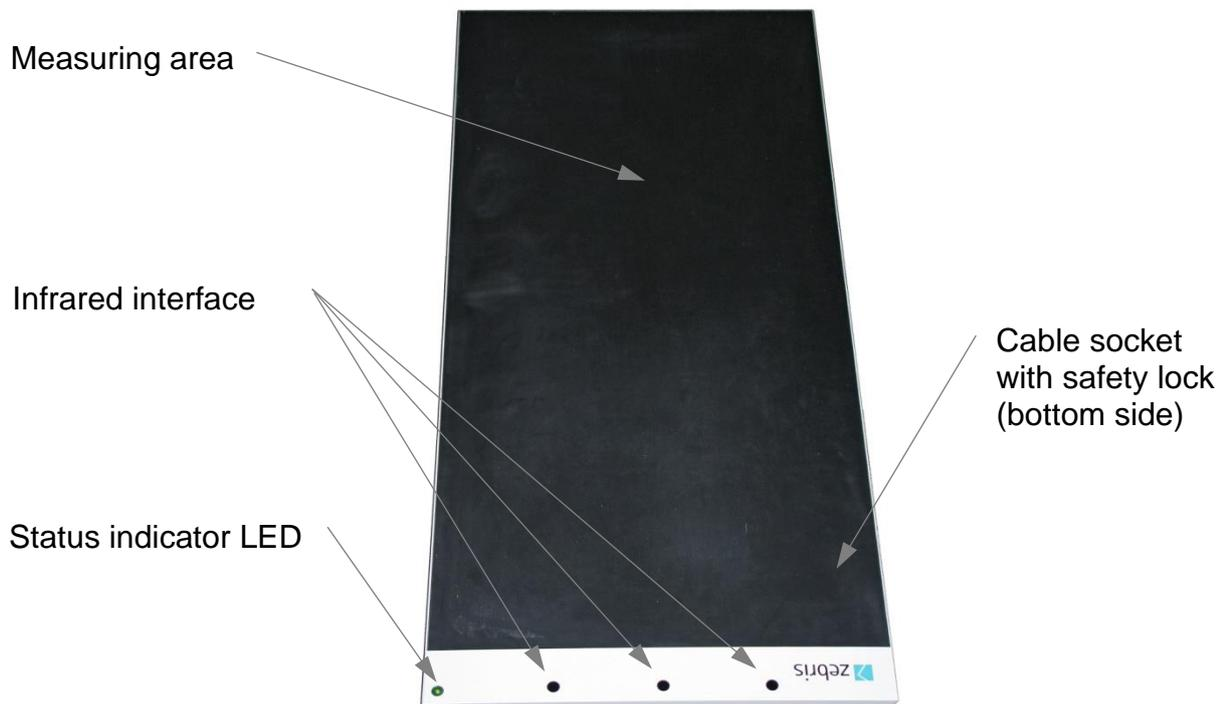
All cable connections between platform and PC will be connected by the cable socket located at the bottom of the platform.
